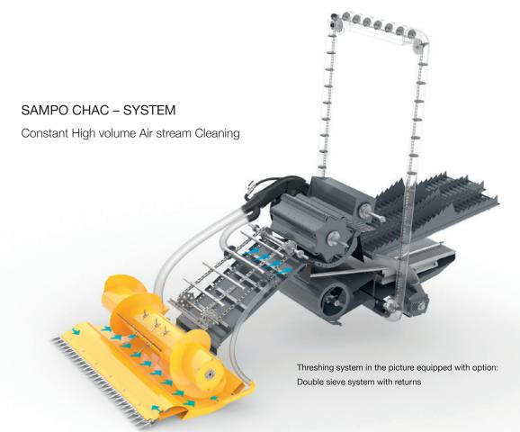
The C2 is equipped with three straw walkers and a single sieve system. The walker area is easy to access from a hatch from the rear. For additional efficiency an optional double sieve system can be fitted on the combine. With the added sieve area, you can choose between 5 different sieves, 5,8,10,12 or 16 mm. The upper sieve is adjustable. This system includes also an efficient return system. The returns are blown back to the grain pan area.
